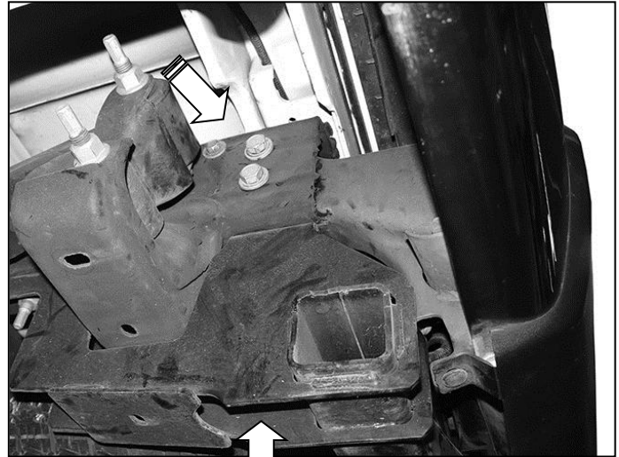
(Fig 2) Remove bumper bolts from side and bottom of frame (arrows) as required
