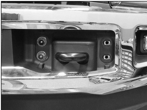
**(Fig 3) Remove outer bumper bolts only**
